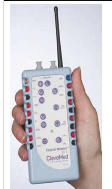
Figure 1 The Crystal Monitor Model 20-S is small enough to be held in the hand and wireless, allowing the sleep patient to get up in the middle of a sleep study without requesting assistance.
