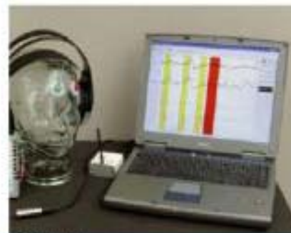
NeuroCAP™ An objective assessment of sleepiness based on the integrated analysis of EEG and task performance.
